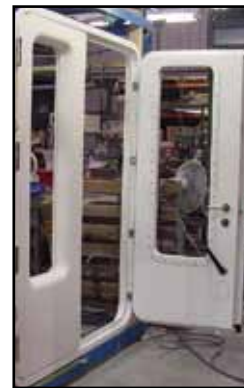
1432 panels configured As 1600 Series, Bi-square actuated concealed dogs
