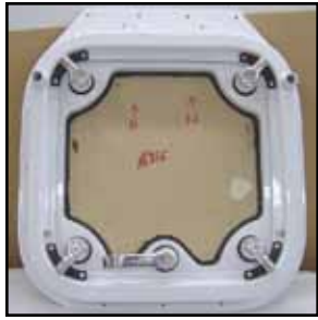
Deep gutter, Underside, Dogged
