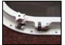
Hinge bolt and deadlight attachment detail
